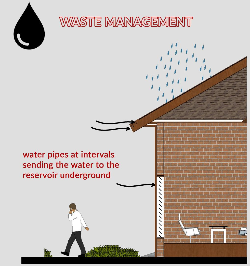
When rain is falling rain water is collected in the two pipes on the roofs and then transported to the reservoir where the water is treated before it is then circulated back to the clinic facility for use in the wash hand basins, laundry and kitchen sinks
