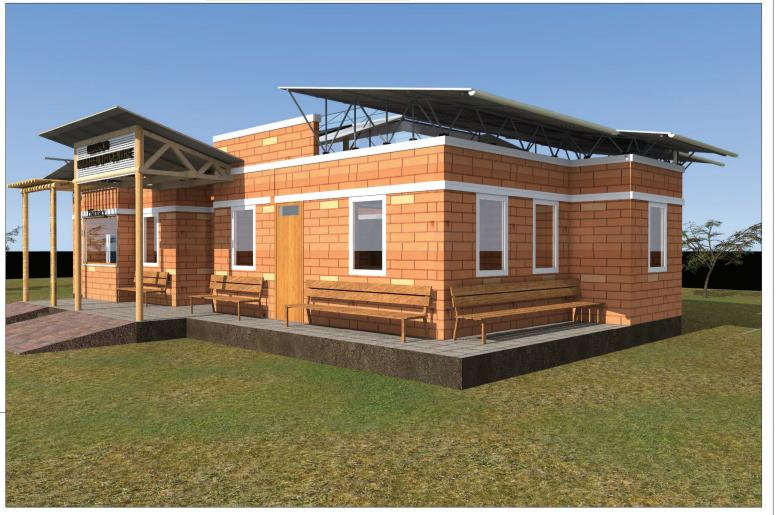
Corrugated iron sheets gauge 28 Sky light for admitting light Solar panels soil blocks (ISSB) Glass casement windows to harwood framing FRONT ELEVATION
