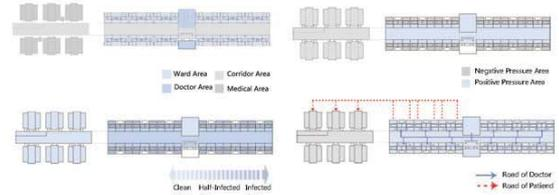
There are 6 medical modules in the medical technology area. With the number 6 as the module to establish the combination system, considering reasonable nursing route, 24 isolation units are combined as a group of isolation ward. To coincide the isolation units, 12 prefabricated bathroom modules are needed. As both the isolation unit and the bathroom module are a quarter of the standard cabin, it will be very efficient in terms of transport.
