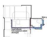
The energy for everyday-life and treatment in the compartment is supplied by the precast equipment box of the shelter hospital. The pipelines are installed below the medical corridor base, attached to each prefabricated bathroom module, and then connected to the compartments on the both sides.
