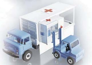
Transfer Track and Forklift for Discharge Isolation Unit
